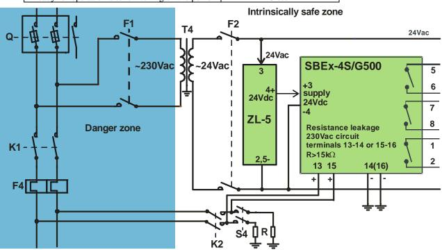
Power supply ZL5 supplier converts 24Vac to 24Vdc which supplies SBEx-4S/G500 separator.
