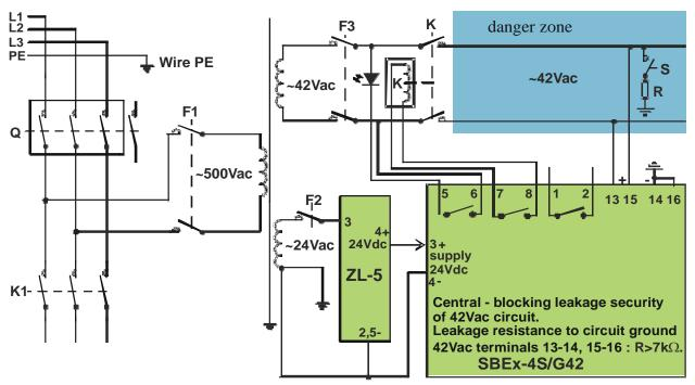
System blocks activation when there is resistance drop in controlled circuit below  $7k\Omega$ . System has three contacts on non-intrinsically safe side confirming that the leakage is below  $7k\Omega$ . Intrinsically safe circuits (terminals 13-14, 15-16) measure leakage in both supply lines 42Vac. There are three non-intrinsically safe output contacts. Contact 7-8 is connected to control circuit K. Contact 5-6 controls signaling circuit.
