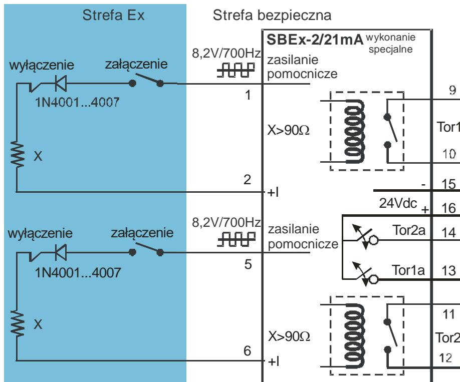
It is possible to order different switching thresholds:  $X > 90\Omega$ , (hysteresis  $17\Omega$ )
