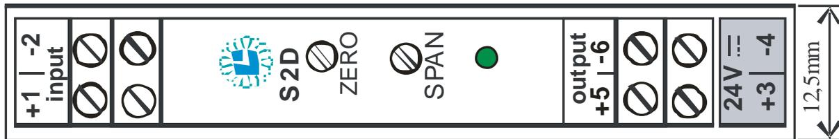
Terminals description for S2D separator with voltage input: S2D-4-?, S2D-5-?, S2D-6?
